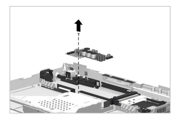
Figure 5-55. Removing the Power Board
